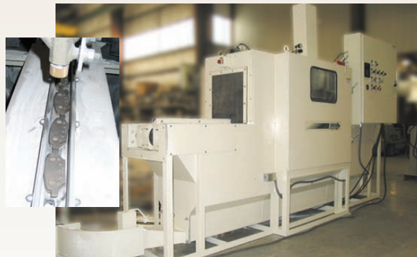
Parts are prepped for paint in a straight-line belt conveyor machine, which is integrated into the production line. This is a fully automated load, blast, paint and drying system.
